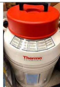
Locator 4 liquid nitrogen tank
